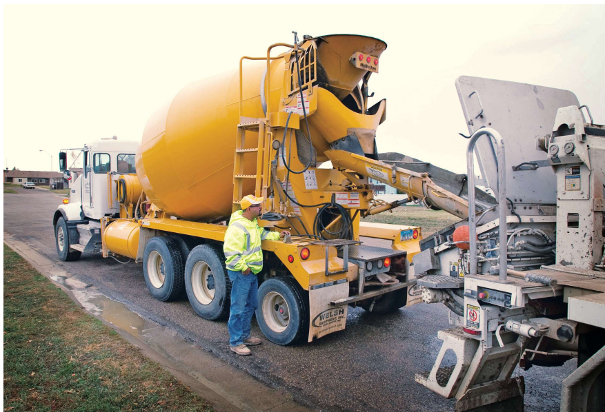
Dickinson driver Andy DeCosteau discharges material into B&W Concrete Pumping's 43-meter Putzmeister concrete pump on a residential project. The concrete will be used by L&D Construction for a foundation on a new housing start.
