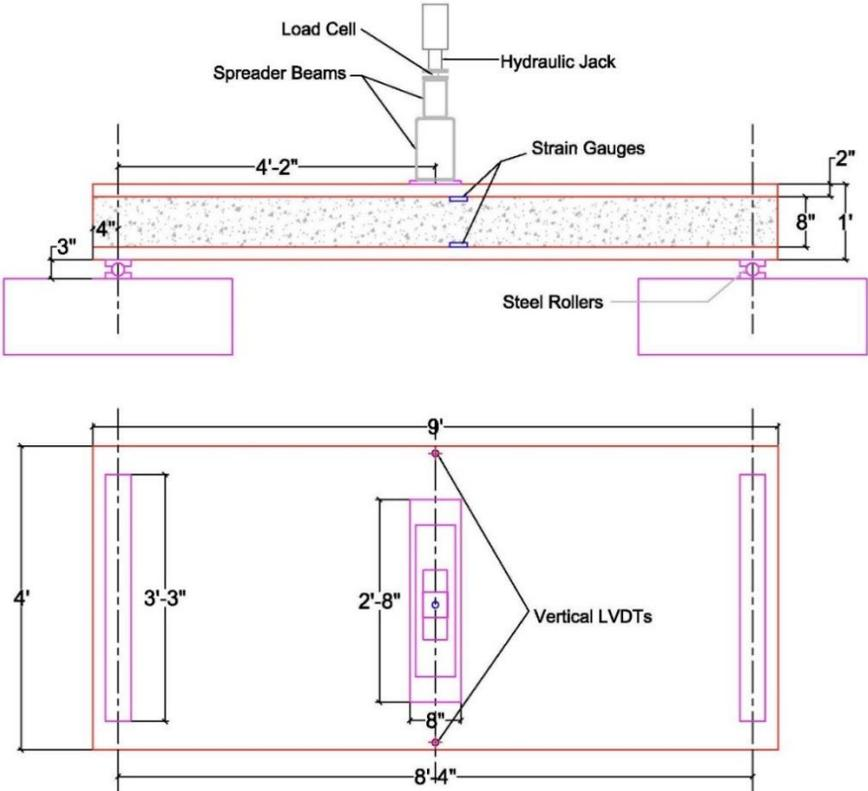
Figure 1: Test setup
