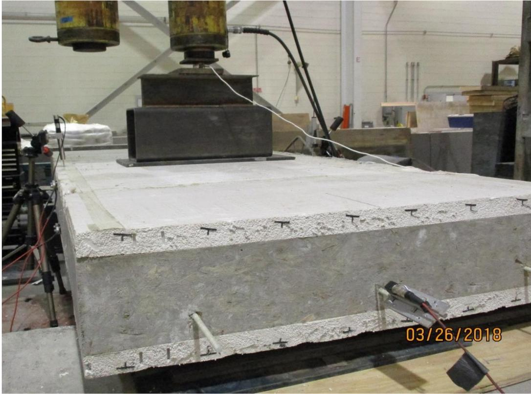
Figure 2: Spreader beams and load cell
