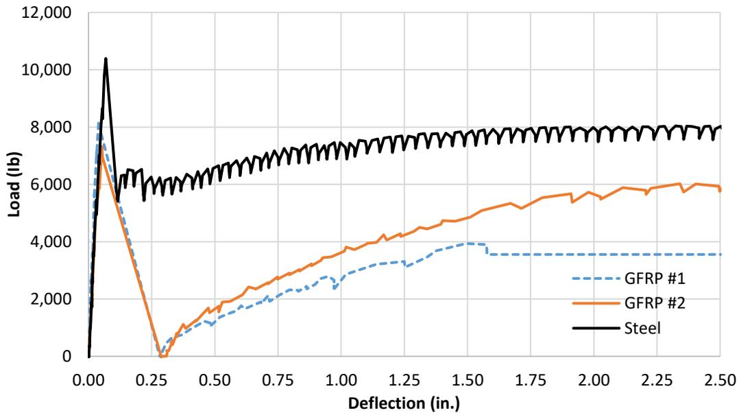
Figure 6: Load-deflection plot for solid wall panels
