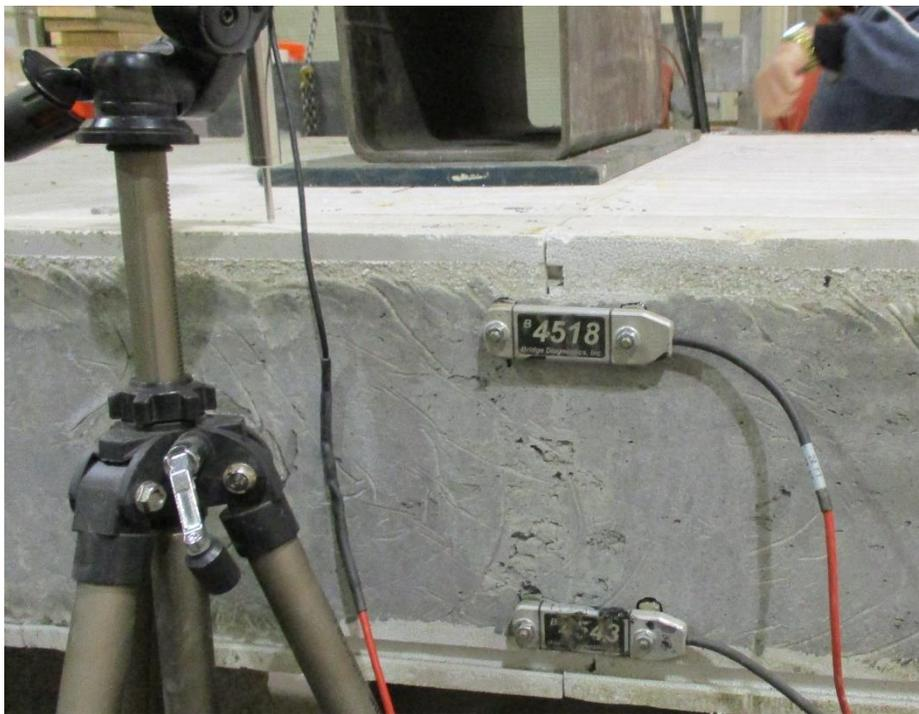
Figure 3: LVDT and strain gauges at mid-span section of the panel
