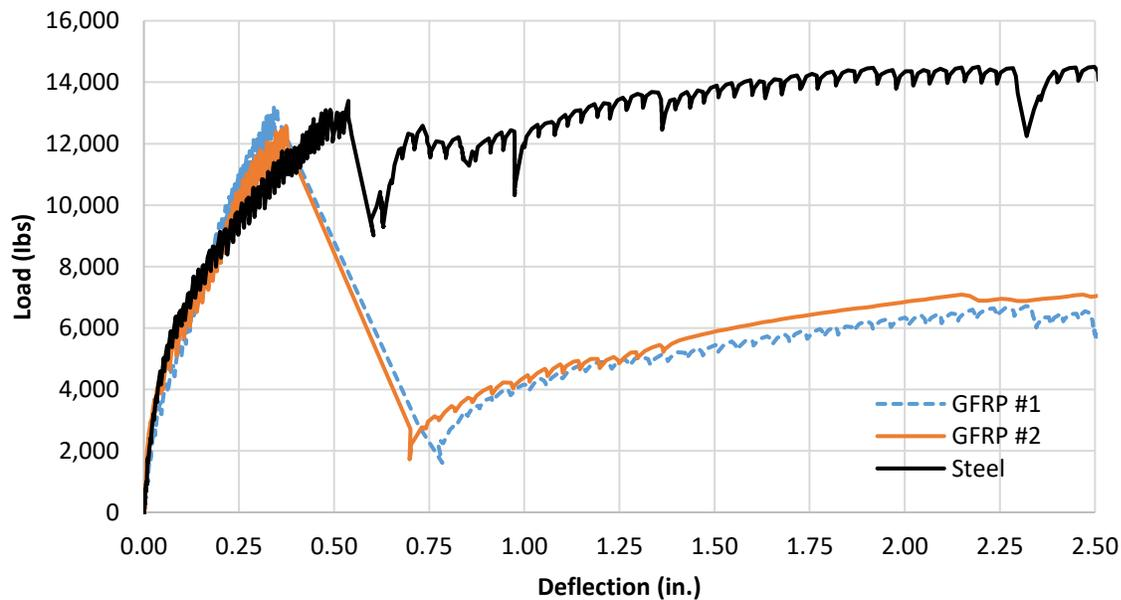
Figure 7: Load-deflection plot for ICF wall panels
