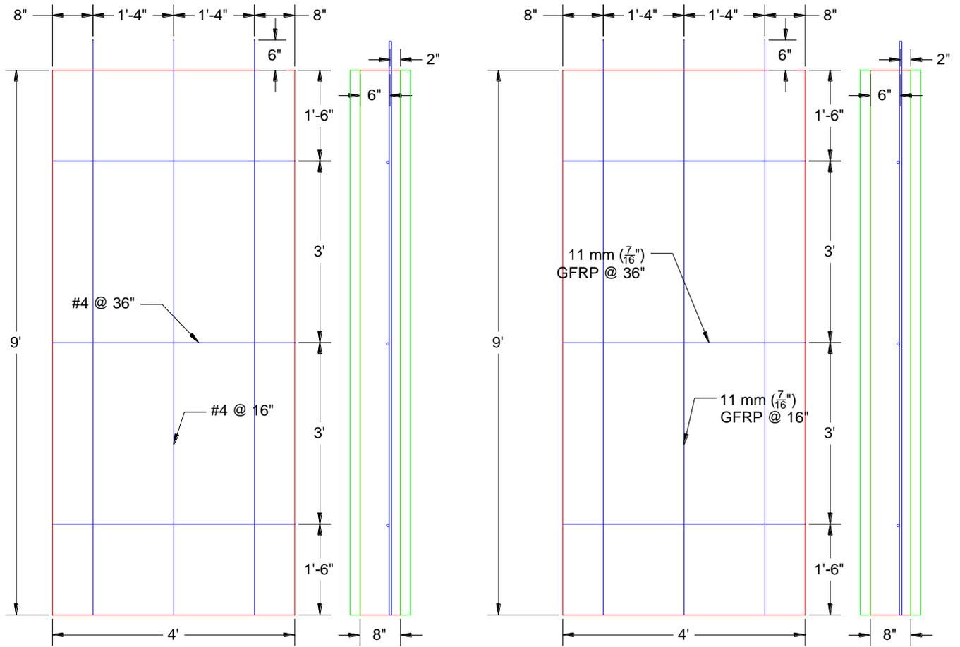
Figure 5: Configuration of the tested ICF wall panels with steel reinforcement (left) and GFRP reinforcement (right)
