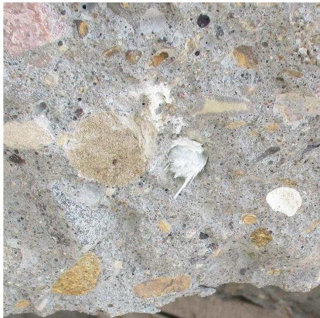
Figure 9: Rupture of GFRP bars
