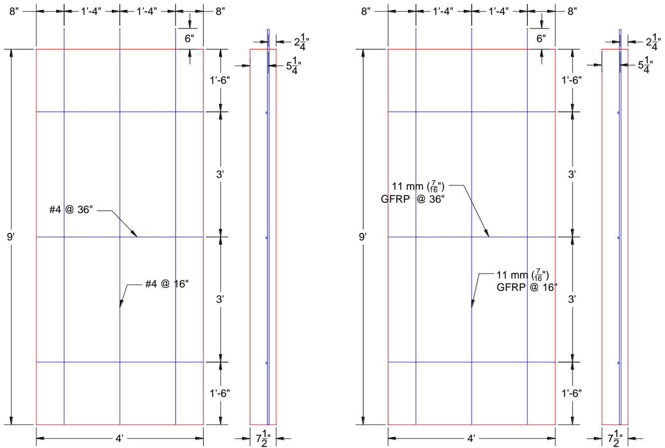
Figure 4: Configuration of the tested solid concrete wall panels with steel reinforcement (left) and GFRP reinforcement (right)
