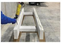
Run 2 long beads of low expansion foam adhesive on each side panel.
