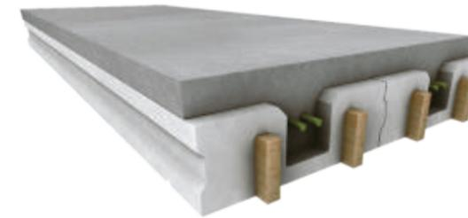
A carpenter friendly wood rib option is available. The wood rib can be removed after placement of concrete to be reused within the construction of the structure. Custom designs and pre-assembly are also options.
