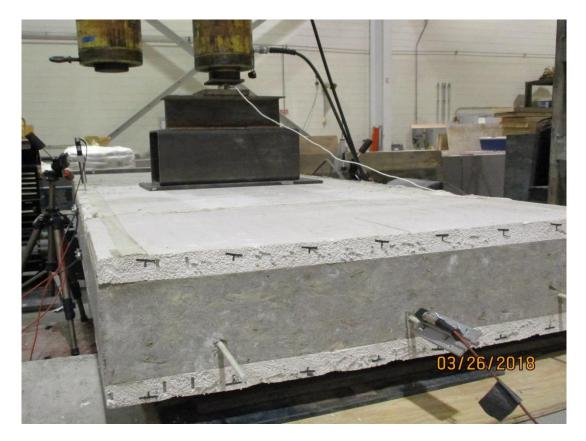
Figure 2: Spreader beams and load cell
