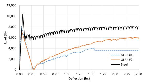
Figure 6: Load-deflection plot for solid wall panels
