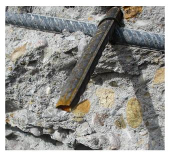
Figure 8: Rupture of Steel bars
