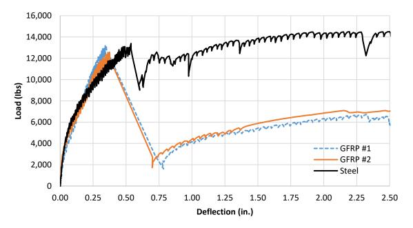
Figure 7: Load-deflection plot for ICF wall panels
