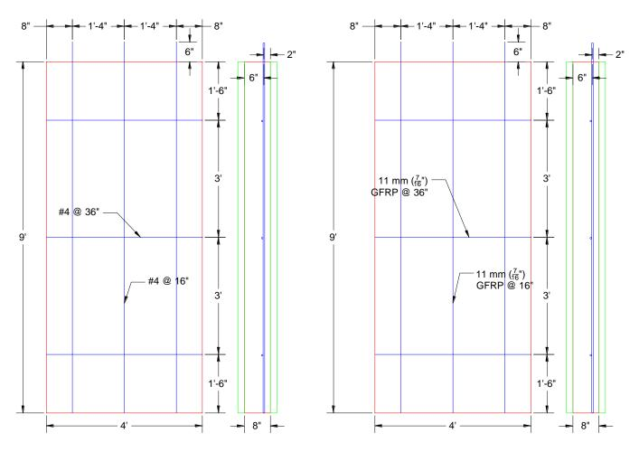
Figure 5: Configuration of the tested ICF wall panels with steel reinforcement (left) and GFRP reinforcement (right)
