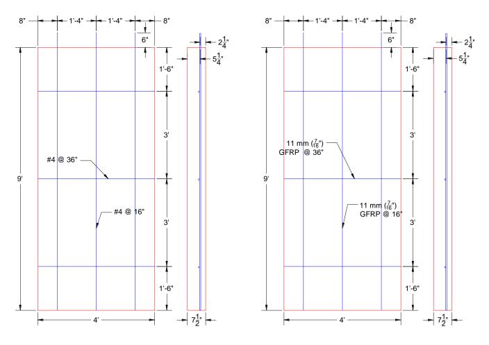
Figure 4: Configuration of the tested solid concrete wall panels with steel reinforcement (left) and GFRP reinforcement (right)
